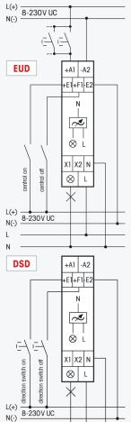
Universal dimmer switch. Power MOSFET up to 400 W. Automatic lamp detection. Standby loss 0.3 watt only. With adjustable minimum brightness, maximum brightness and dimming speed. With switching operation for children's rooms and snooze function.
