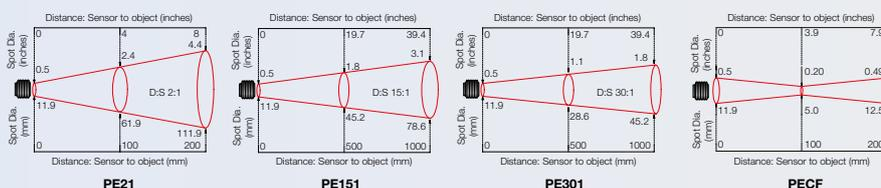
All PyroEpsilon sensors are fitted with precision Germanium lenses for accurate optics. Model PE21 has 2:1 optics making it suitable for most applications where the sensor can be mounted close to the target. Model PE151 is designed for small or distant targets and has an optical resolution of 15:1. Model PE301 is designed for very small or distant targets and has an optical resolution of 30:1. Model PECF is designed for targets as small as ø5 mm at a distance of 100 mm from the sensor
