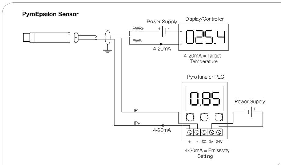
The PyroEpsilon Series is a range of high quality, low cost, compact sensors which measure the temperature of inaccessible or moving objects and materials. They measure temperatures from -20°C to 500°C, accurately and consistently, with an outstanding response time of 240 ms.
