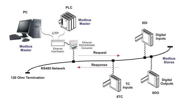
Fig: Max. 4 masters can access data of the IO modules via PC-E in Mode 0. That means Mode 0 supports multi socket communications.
