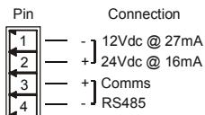
Note: If power/communication connections are reversed, module may become faulty.
