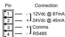
Note: If power/communication connections are reversed, module may become faulty.
