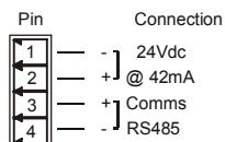
Note: If power/communication connections are reversed, module may become faulty.
