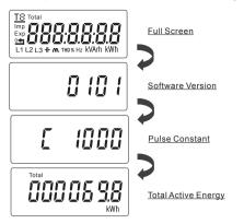
The default display is total active energy kWh for EM3-100, EM3-100-R; while import active energy for EM3-100-Bi.
