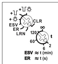
**With the top rotary switch** in the setting LRN up to 35 wireless pushbuttons can be assigned therefrom one or more central control pushbuttons. In addition wireless window/door contacts with the function N/O contact or N/C contact while the window is open, wireless outdoor brightness sensors FAH and wireless motion/brightness sensors FBH. The required function of the impulse switch with integrated relay function can then be selected:
