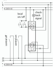
1 NO contact + 1 NC contact potential free 16 A/250 V AC. Incandescent lamp load up to 2000 W.
