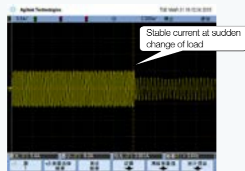
Current waveforms when sudden unloading in V/F control mode with 2Hz and full load
