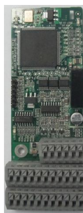
UVW incremental PG card EC-PG503-05
