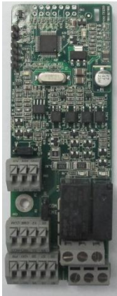
IO extension card EC-IO501-00
