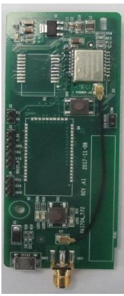
Bluetooth communication card EC-TX501/502
