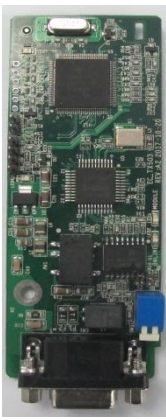
PROFIBUS-DP communication card EC-TX503
