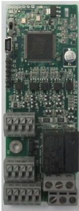
PrPogrammable extension card EC-PC501-00
