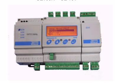
The gas detection central unit CE100R, is a DIN rail realization, is composed by a central unit for the electronic data elaboration, a display 122 x 32 points back lighted with key board and connectors for the power supply from 20 to 30Vcc, for the input of the detectors' information, for the alarm output and for optional equipments.
