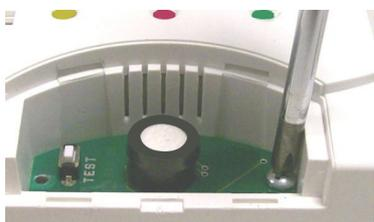
2 • Undo the two screw fasteners on the Sensor module to be replaced. (Fig. 12).
