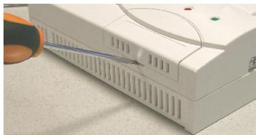
1 • Turn off the detector, unplug it from the mains and use a screwdriver to lever off the little cover under the three LEDs (Fig. 11).
