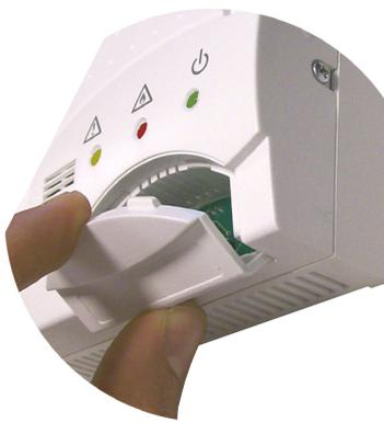
5 • Fasten the **Sensor module** with the two screws and close the cover, first inserting the two tabs at the bottom (Fig. 15). The instrument can now be turned on.
